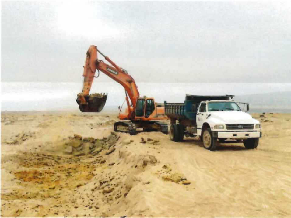
Mining method on site – simple truck and shovel – extracting product at near surface
